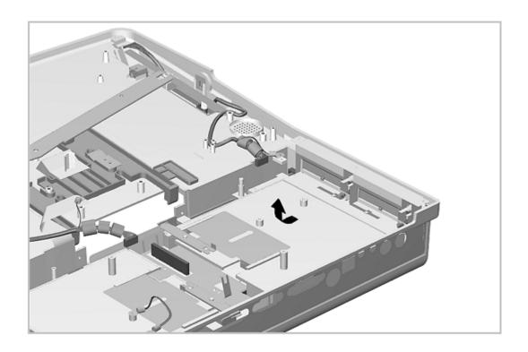
Figure 7-23. Removing the MultiBay Assembly
